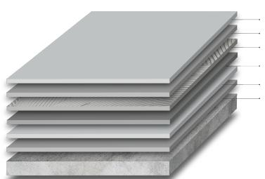
**Application of 2<sup>nd</sup> Topcoat:** Polyurethane 100/100 VOC
