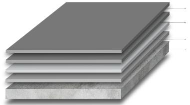
Static Dissipative Finish Coat: Stat-Rez® ESD Nano 275
